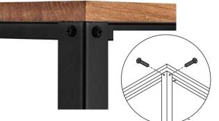
Step One:Install the four metal frame to the MDF board.
