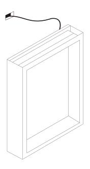
When Doors facing you, the electrical wire comes out through the access hole in the **TOP RIGHT SIDE** of the cabinet.
