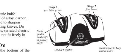
Your Presto<sup>®</sup> EverSharp<sup>™</sup> electric knife sharpener will sharpen knives of alloy, carbon, or stainless steel. It is designed to sharpen kitchen knives and most sporting knives. Do not attempt to sharpen scissors, serrated electric knives, or any blade that does not fit freely in the blade guides.
