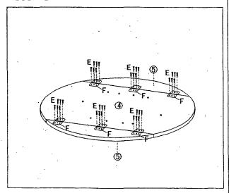
Assemble top panel (4) and dropped table leaves (5) together by using screw (E) as shown.
