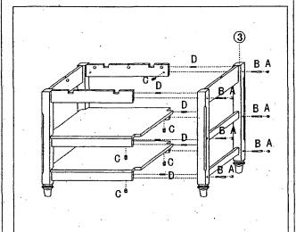
Assemble side frame (3) to step 2 assembled unit by using camlock bolt (B),camlock (C) and wooden dowel (D) as shown. Then plug in plastics cover (A) to holes as shown.
