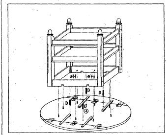
Assembled table top unit to step 3 assembled unit by using wooden dowel (D) and camlock (H) as shown.
