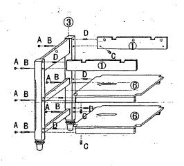
Assemble top apron (1) and\_step one assembled unit to side frame (3) by using camlock bolt (B),camlock (C) and wooden dowel (D) as shown. Then plug in plastics cover (A) to holes as shown.
