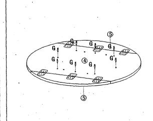
Screw camlock bolt (G) to back of table top (4) as shown.
