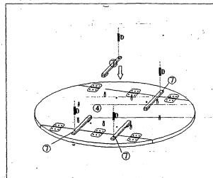
place extension rail (7) onto back of table top (4) as shown. (D) and camlock
