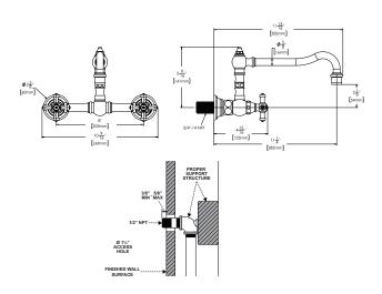
1. All dimensions are in inches (millimeters) unless otherwise specified and are subject to change without notice. 2. Contractor to supply necessary inlet connections.
