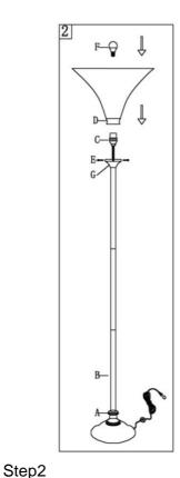
Put the shade(D) into the CUP(G), then tighten three screws (E) into the CUP (G) Insert the bulb(F) into the socket(C).
