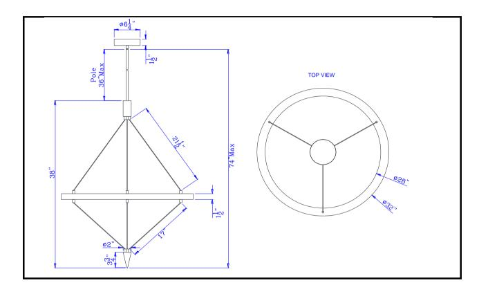
Description: Integrated dimmable LED wood pendant fixture with suspended steel braided wire. 24W,
