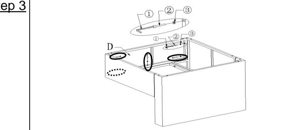
Attach Side Plate(D) between the Back(I) and Seat(J) using Bolt(2) and Washer(3) with Allen Key(1) as shown above.
