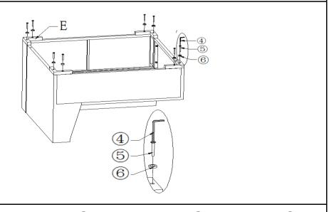
Attach the Foot(E) to the Chair using Bolts(5) and Washer Rings(6) with Allen Key(4).
