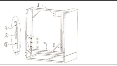
Attach Seat(J) between the Left Armrest(H) and Back(I) using Bolt(2) and Washer(3) with Allen Key(1) from position # I to # V as shown above.
