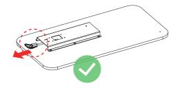
The handle should be near the edge of the desk board as shown.
