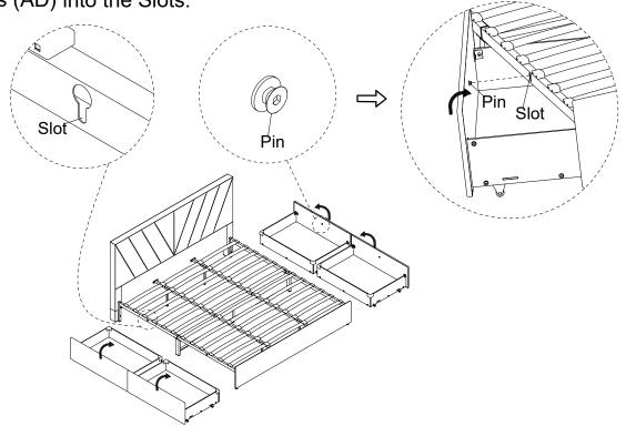
When pull out the drawers, lift the drawers first in order to make the Pins released from the Slots freely, then pull the drawers toward outside. DO NOT PULL OUT THE DRAWERS DIRECTLY.
