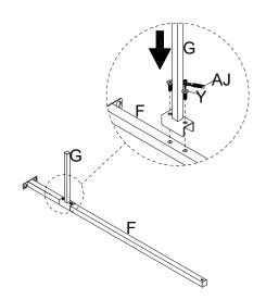
Attach the Center Rail - Front / Rear (F) to the Headboard (A) and the Footboard (B), insert the Bolt (Y), turn the Ratchet Tool (AJ) to tighten them. Then attach the Center Rail - Front / Rear (F) to the Center Support Bar (C), insert the Bolt (Z), turn the Ratchet Tool (AJ) to tighten
