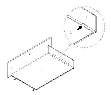
Insert another Drawer Side Board (I) to the Drawer Bottom Board (L) first, and attach the Drawer Side Board (I) to the Drawer Bottom Frame (K), then insert the Bolt (AA) and Washer (AG), turn the Ratchet Tool (AJ) to tighten them.
