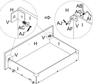
Insert the Bolt (AD) and Washer (AG) to the back of Drawer Front Board (H), turn the Ratchet Tool (AJ) to tighten them.
