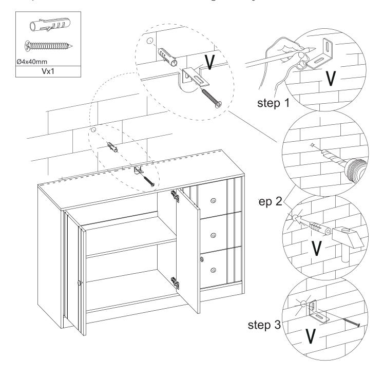
If it is a solid wall, please use expansion and self-tapping screws to secure the cabinet to the wall, if it is a wooden wall, only use self-tapping screws. Please dont overtighten screws.
