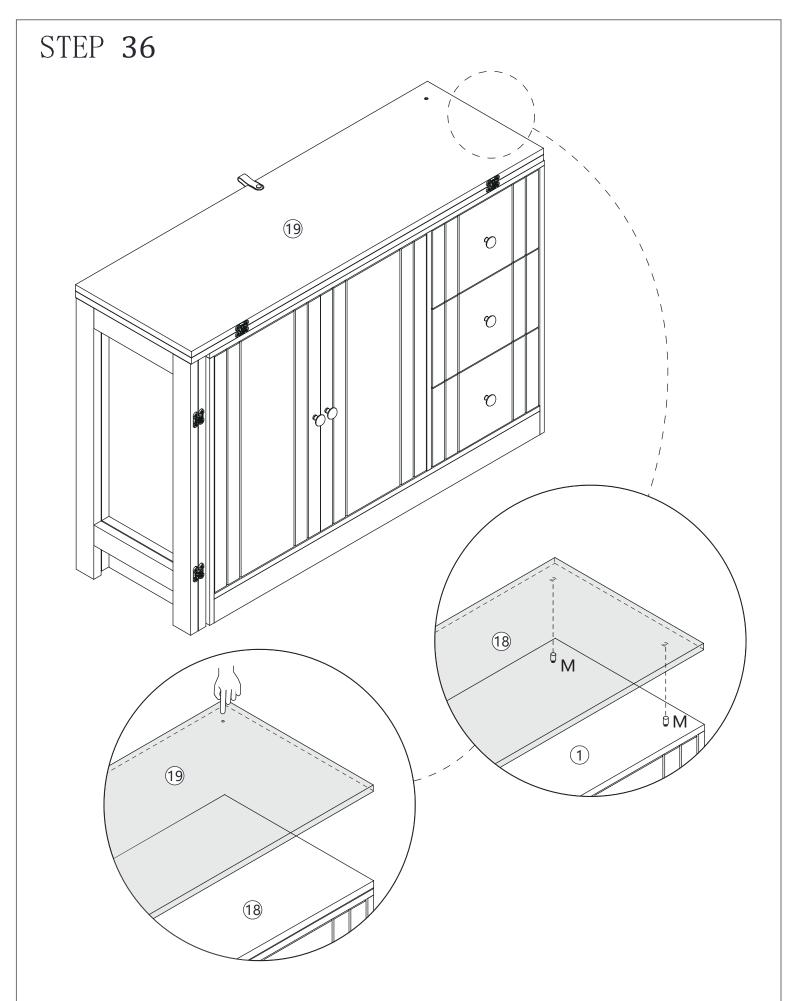
Align the holes on Panel (18) with M on Panel (1). After folding the table, the hole on panel (19) will face upward.
