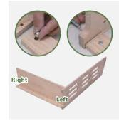
① Position Frame (a), Bottom Slat (i), and Bottom Panel (n) as picture shown. Secure with Flat Head Screws (r).
