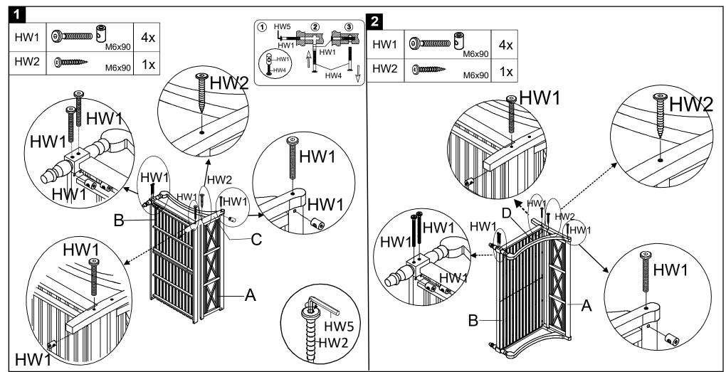
**Step 1**: Attach the Back (A) and the Seat (B) to the Left side (C) by using the T bolt & nut (HW1) and the Screw L (HW2) as shown on the picture. Tighten it with the Allen key (HW5).
