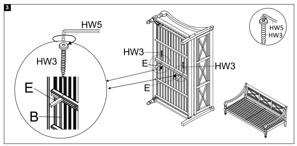
Step 3: Attach the Support seat (E) to the Seat (B) as shown on the picture. Using the Screw (HW3) to fit and tighten by the Allen key (HW5).
