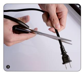
The second method of use is to use a tool to cut off the plug and separate the neutral and live wires.
