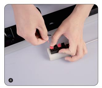
Connect the wires on the light to the corresponding neutral wire, live wire and ground wire, and put them in the wire box for insulation protection.
