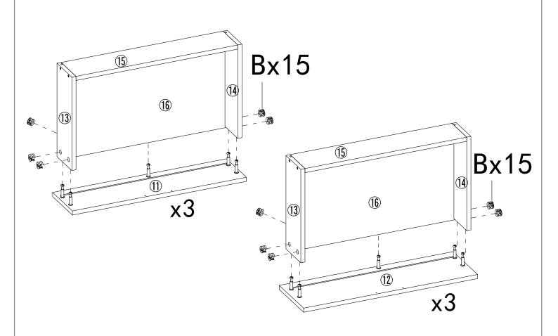
Connect panel 11 to panel 13&14 with hardware B. Connect panel 12 to panel 13&14 with hardware B.
