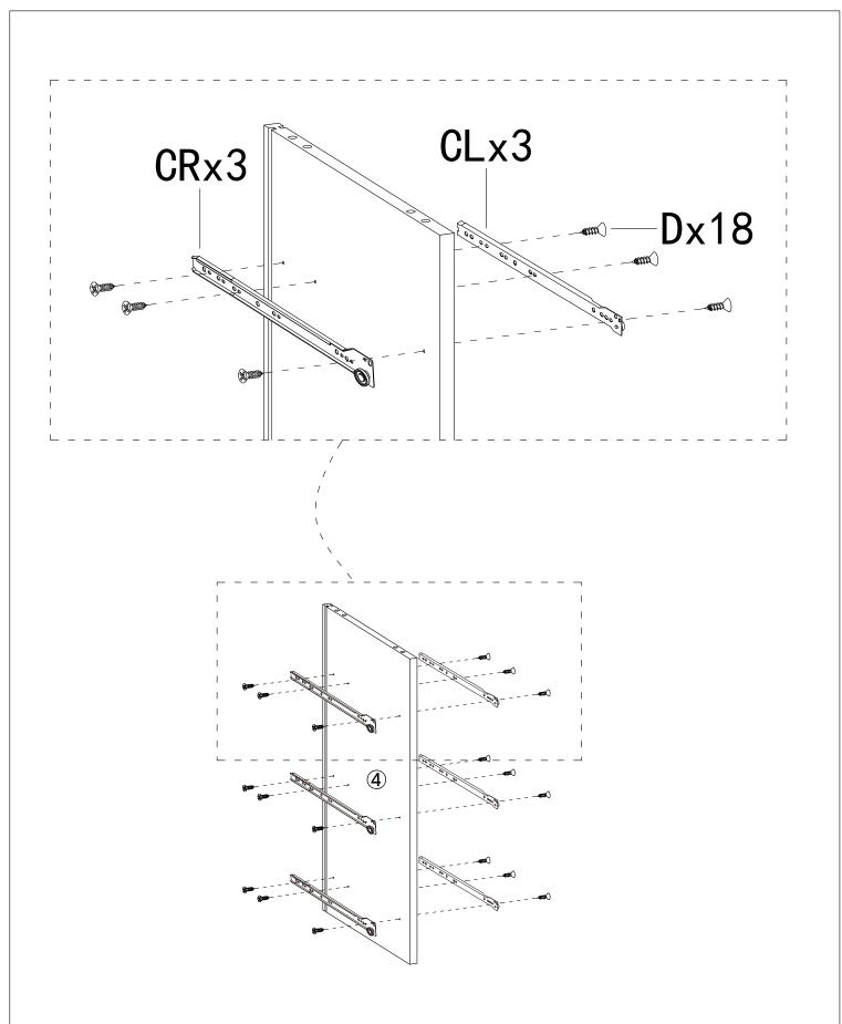
Fix sliding rail CL and CR to the both sides of panel 4 with screw D.
