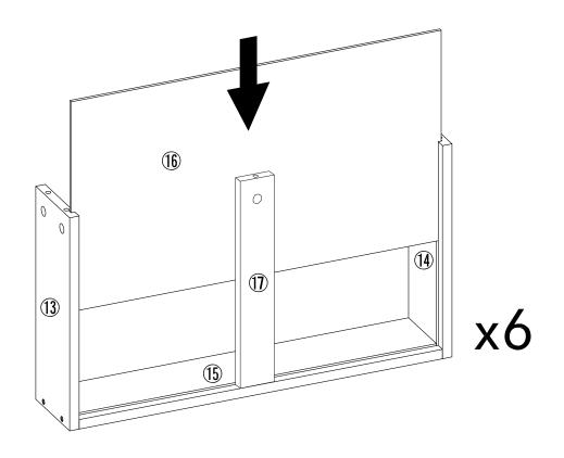
Insert panel 16 into the slot.
