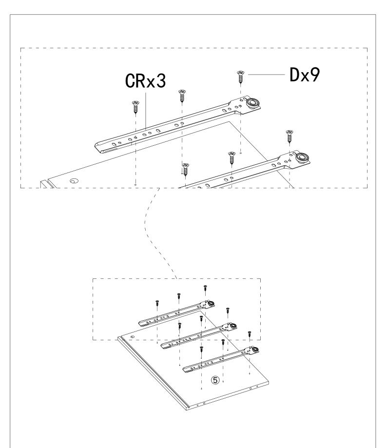
Fix sliding rail CR to panel 5 with screw D separately.
