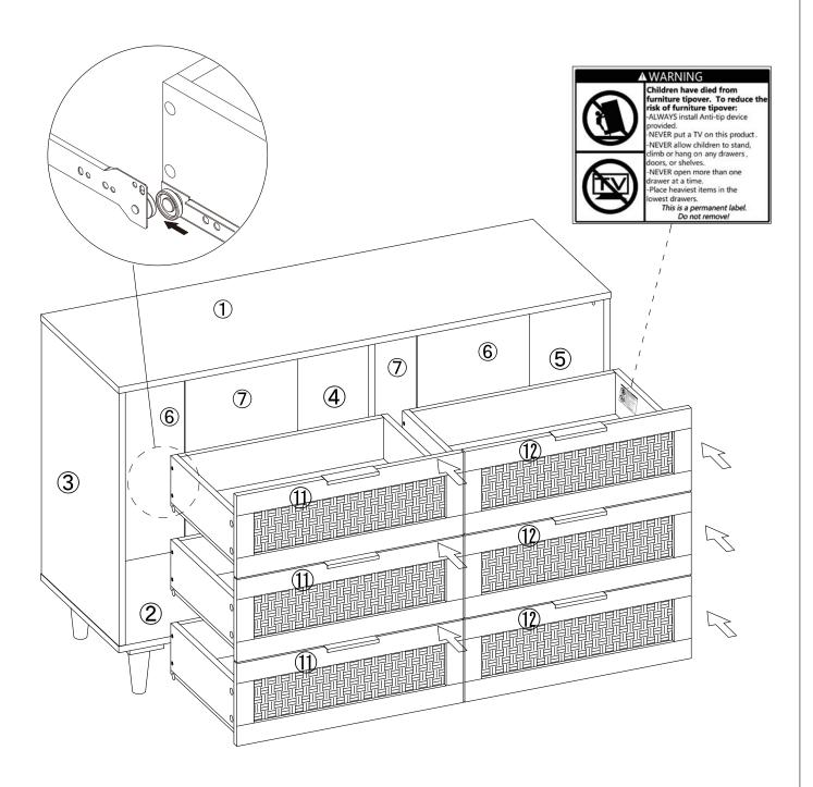
Drawer with panel 11 must be put on the left, drawer with panle 12 must be put on the right, otherwise, they will be not ifx well.
