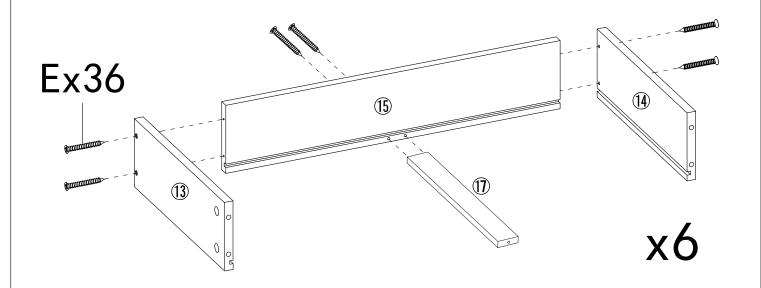
panel 13 to panel 15 with screw E. panel 14 to panel 15 with screw E. panel 17 to panel 15 with screw E.
