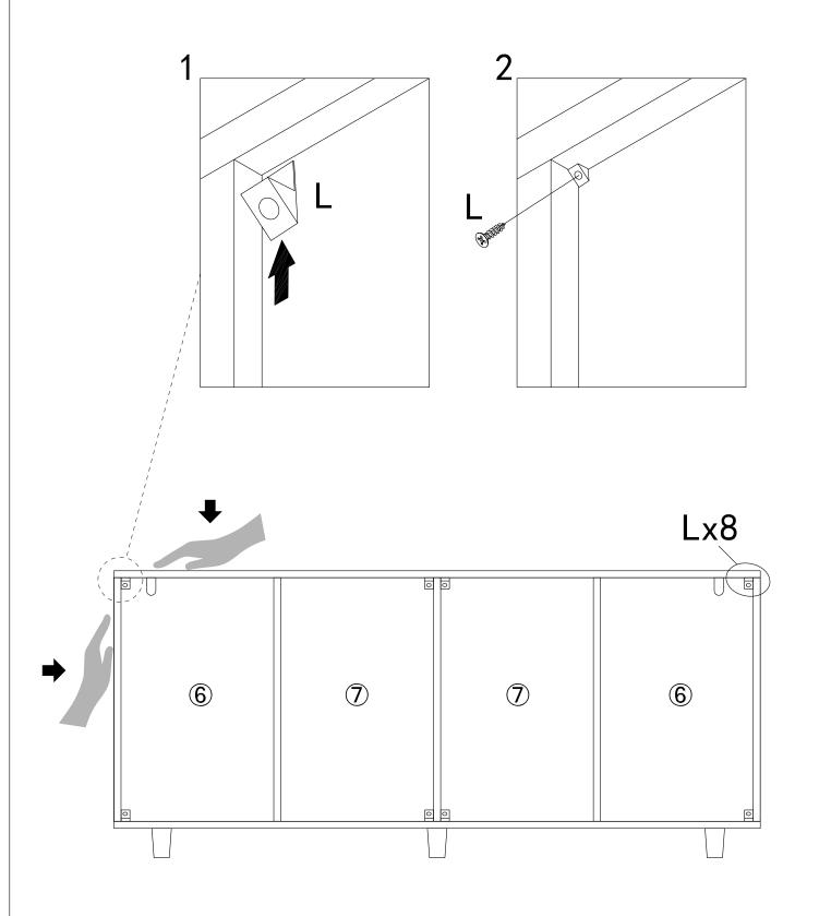
step 1.Mark the position on the wall. step 2.Drill and insert the expandable screw Lby hammer. step 3.Use screw E to attach it and tighten by screwdriver.
