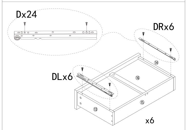
Fix sliding rail DL to panel 13 with screw D separately. Fix sliding rail DR to panel 14 with screw D separately.
