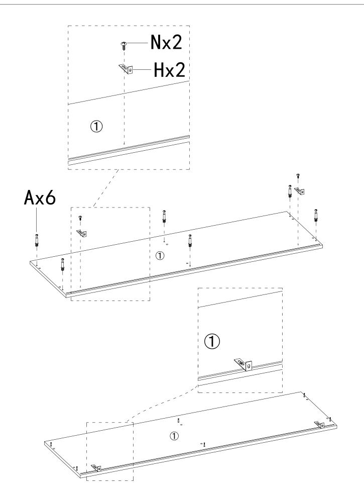
screw A to panel 1, connect hardware H to panel 1 with screw N.
