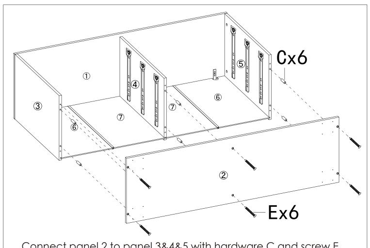
Connect panel 2 to panel 3&4&5 with hardware C and screw E.
