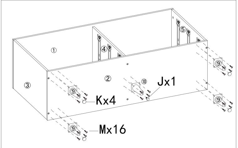
Connect hardware 9&10 to panel 2 with screw M. rew hardware K to panel 9, then screw J to panel 10.
