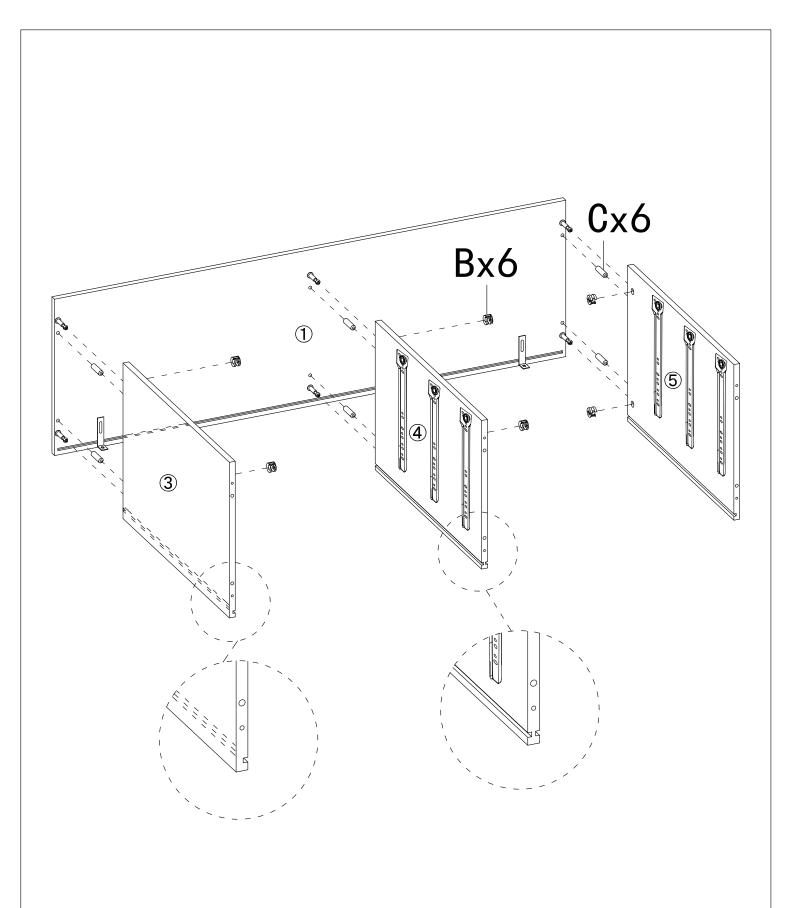
the slot of panels are downward. connect panel 1 to panel 3&4&5 with hardware B and C.
