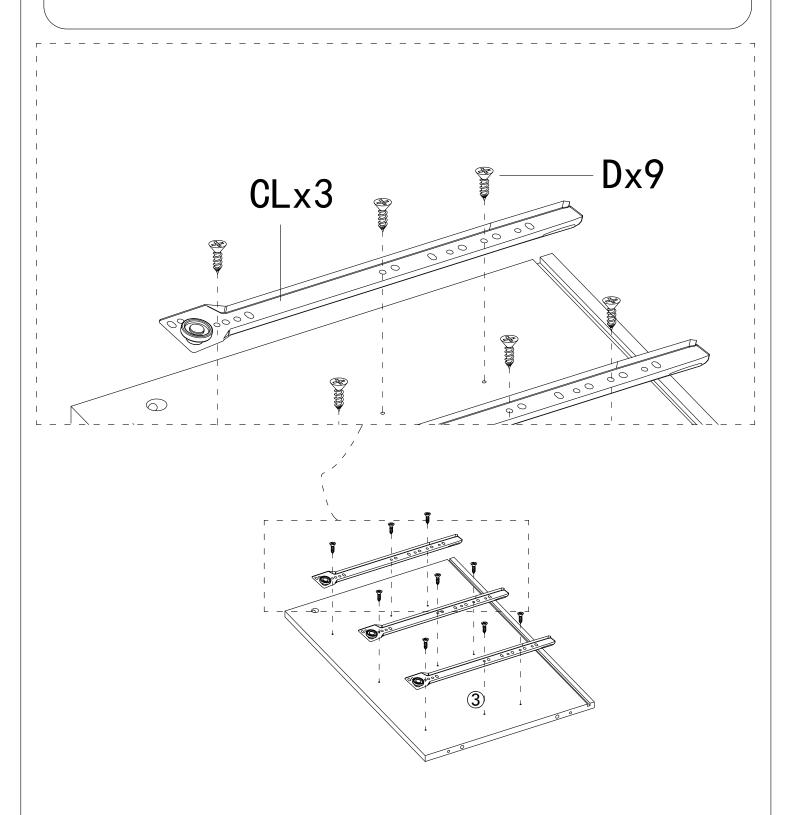
Fix sliding rail CL to panel 3 with screw D separately.
