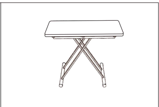
STEP3: Pull up the lifting adjusting wrench and lift the table top upward to improve the height of the table.
