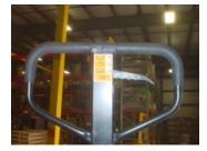
Lower - lever up (lever moves back to drive position when released)
