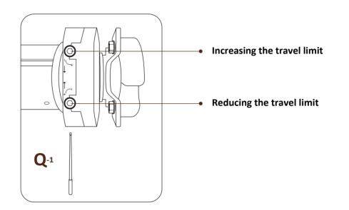
According to motor rotating direction, adjust the travel limit with the use of the 4mm hex wrench #Q-1.
