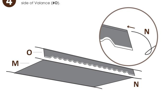
Thread three Guiding Wires (#N) through both ends of the large Fabric (#M) and
