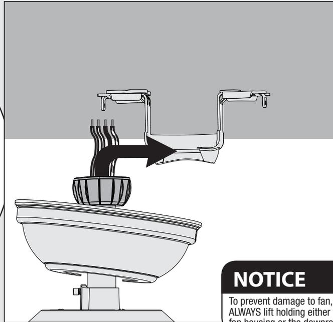
Place the downrod ball into the slot in the ceiling bracket.
