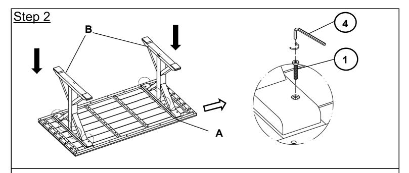
Attach the Legs(B) to Table Top(A) using Bolts(1) with Allen Key(4) as pictured. Do not fully tighten the Bolts.
