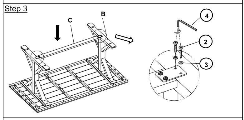
Align Leg Support Bar(C) between Legs(B) as shown above.
