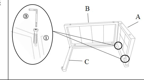
Attach the Top Panel(A) to Right Side Support Bar(C) and Side Panel(B) using Bolts(1) with Allen Key(3) as shown above.
