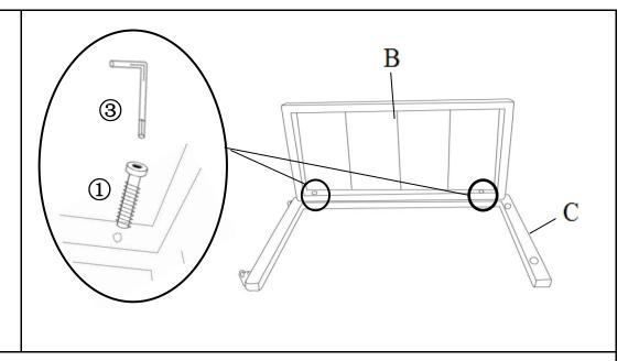
Attach the Side Panel(B) to Right Side Support Bar(C) using Bolts(1) with Allen Key(3) as shown above.
