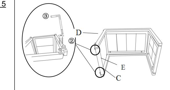
Attach the Horizontal Base Support Bar(E) to Right Side Support Bar(C) and Left Side Support Bar(D) using Bolts(2) with Allen Key(3) as shown above. **Do not fully tighten Bolts.**
