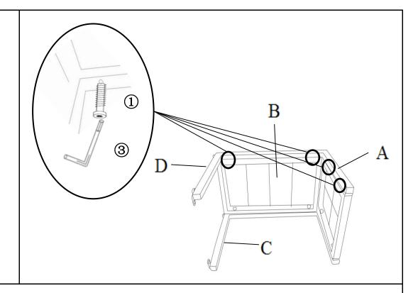
Attach the Left Side Support Bar(D) to Top Panel(A) and Side Panel(B) using Bolts(1) with Allen Key(3) as shown above.
