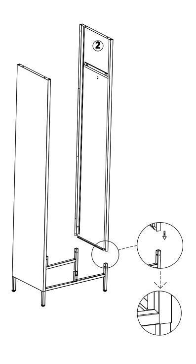
Step 4: Fix 1, 2 and 3 with screws A
