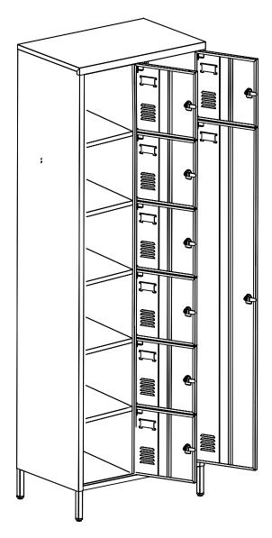
For the bottom two doors: Insert the door pivots E into the holes of the right bottom corners(shims F can be used to adjust, you can use 0/1/2 of them), then insert the doors into the door pivots on the bottom and adjust the springs (already pre-installed) on the right top corners For the other doors: Insert the doors into the lower doors' spring pivots of the right bottom corners and adjust the springs on the top So only two E are needed
