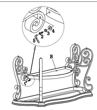
STEP 2: Attach Shelf (B) to Legs( E) by using Allen Key M4 (5),Allen Bolt 1/4"x28mm (2), Spring Washer 1/4" (3), Flat Washer 1/4" (4)
