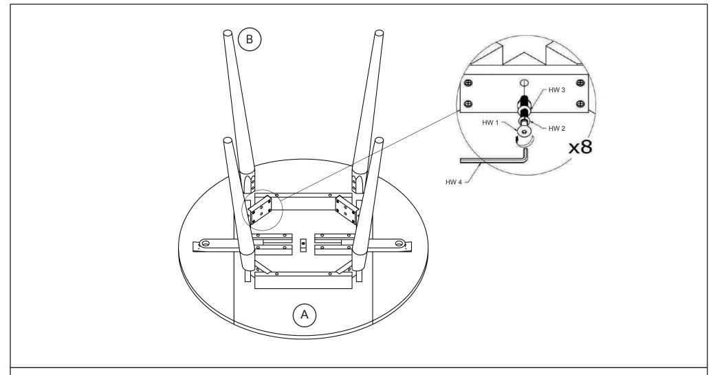
**Step 1 :** Place the table leg (B) in position and screw in the bolts (HW1). Put the washer (HW2,HW3) on the bolts (HW1) in the order shown in the picture.
