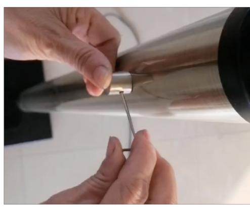
STEP 2: Insert a 0.2mm Allen wrench and tighten until snug. Do not overtighten.
