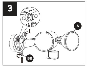
Attach the light fixture (A) to the mounting plate using the mounting plate screw (FF). Then insert the rubber plug (DD).
