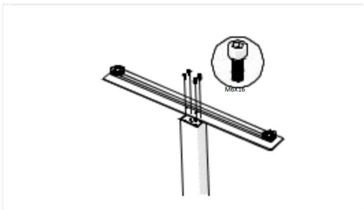
Step 5: Install the desk legs according to the instructions above. Press the smooth side of the tabletop against the desk legs. Please refer to the screw list to select the appropriate support feet and matching screws. Please refer to the torque guide.
