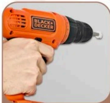
Drill Anchor into Wall
