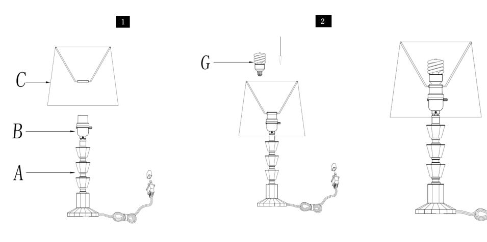
Step 1 Unpack all parts from cartons carefully Put the shade(C) on the Socket(B), then
