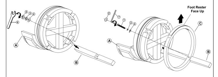
**Step 2:** Attach Leg (B) to the Chair Back (A) by using Flat Washer (4), Lock Washer (3), Hex Nut (5) and secure by Wrench (6). Insert Flat Washer (4), Lock Washer (3), Bolt (1) into the holes of the Hoop (C) to attach with Leg (B) and secure by Allen Key (7). Fully tighten all bolts at this time. Insert the Plastic Cap (2) into the holes of the Hoop (C). Assembly product is now completed.
