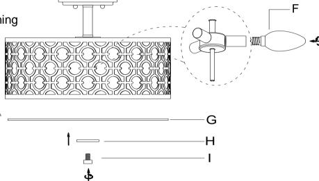
PLEASUE USE TYPE"B" BULB MAX 40-WATT OR CFL BULB MAX 9-WATT THERE ARE 3 X 25W BULBS IN THE BOX.
