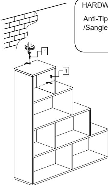
**NOTE :** Wall fixings are not supplied with this product as different wall materials require different types of fixing devices (such as Rawl plugs on brick work). You must use fixing devices suitable for the type of wall you intend to mount this product to. Please ensure that the head of any screw used has a diameter greater than the diameter of the mounting hole on the bracket and that the fixing is safe and secure before use. The screw supplied is to fix the anti-tip strap to the shelf.
