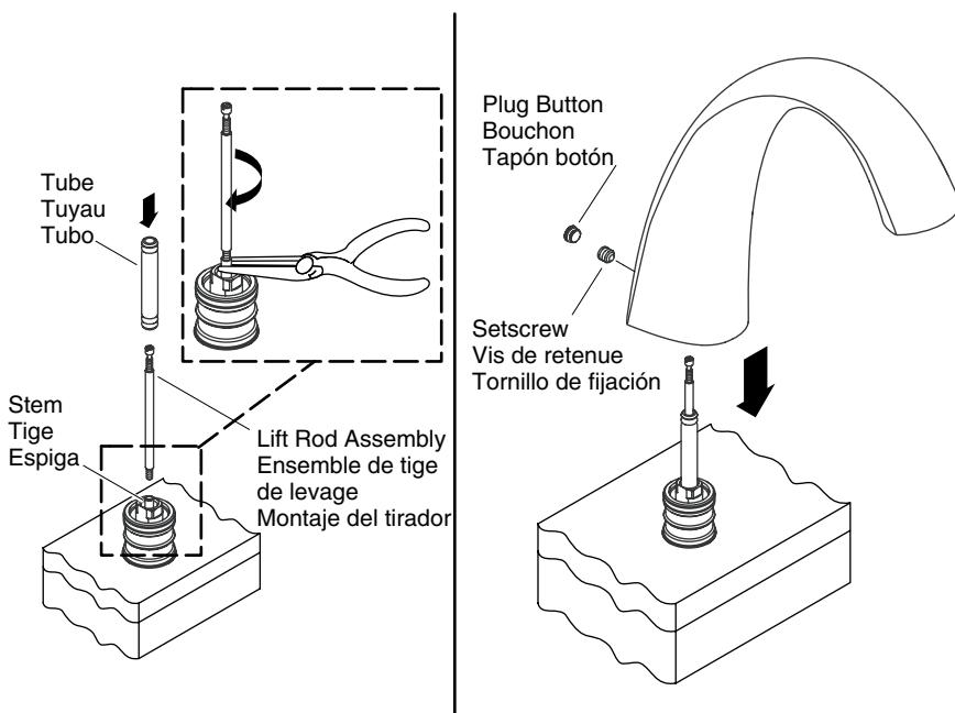
**NOTICE:** To avoid damage to the O-rings while assembling the spout, ensure the diverter body and tube are clean.
