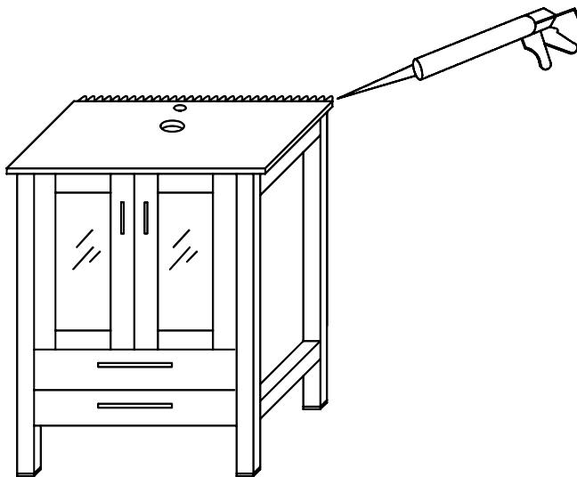
To help prevent mildew, apply sealant to the space between the wall and the edge of the cabinet.
