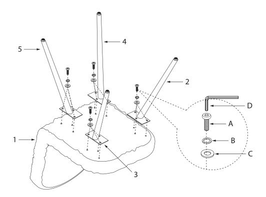
FULLY TIGHTEN ALL BOLTS USING ALLEN WRENCH (D).
