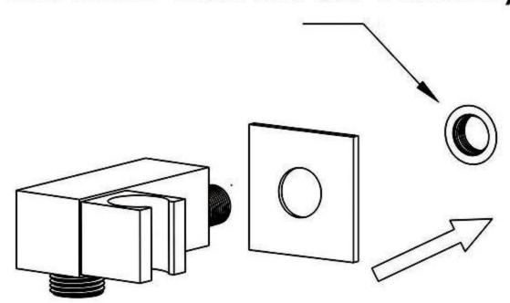
6.Install body jets (Wrap the PTFE) tape on the thread)
