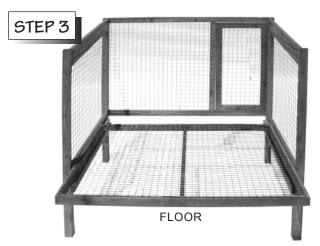
Slide Floor into Bottom of Hutch, Wire Side Up. Align Side Holes and Fasten Back Panel (**D**) to Side Panels using **6**- 1 1/2" Bolts and **6**- Wing Nuts.
