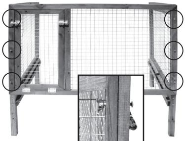
Fasten Side Panels (B) to Front Panel (C). Use 6- 2 1/4" Bolts and 6- Wing Nuts.
