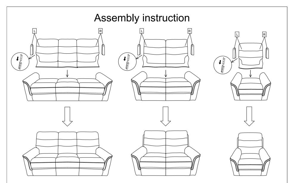
STEP 1. Hold up the Backrests, while standing behind, insert the small metal arms on the under-insides of the Backrest into the prefabricated slide lock gadget on the Seat Base, push the Backrest downwards until the Backrest is fully slotted and locked into position.
