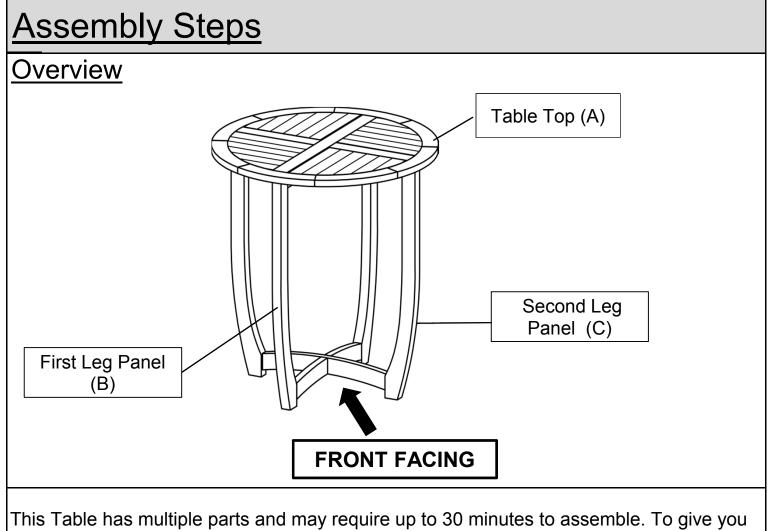
an overview of the Table parts, the above picture is to help you put the various parts into perspective. Please read through the instructions below to familiarise yourself with the parts and steps before assembly.
