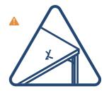
6. Pay attention to avoid over-tightening fasteners, or they may induce cracking within the board.
