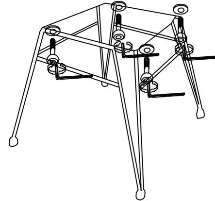
2.Assemble the table leg(C) to the table top(D),using bolt and washer(F).
