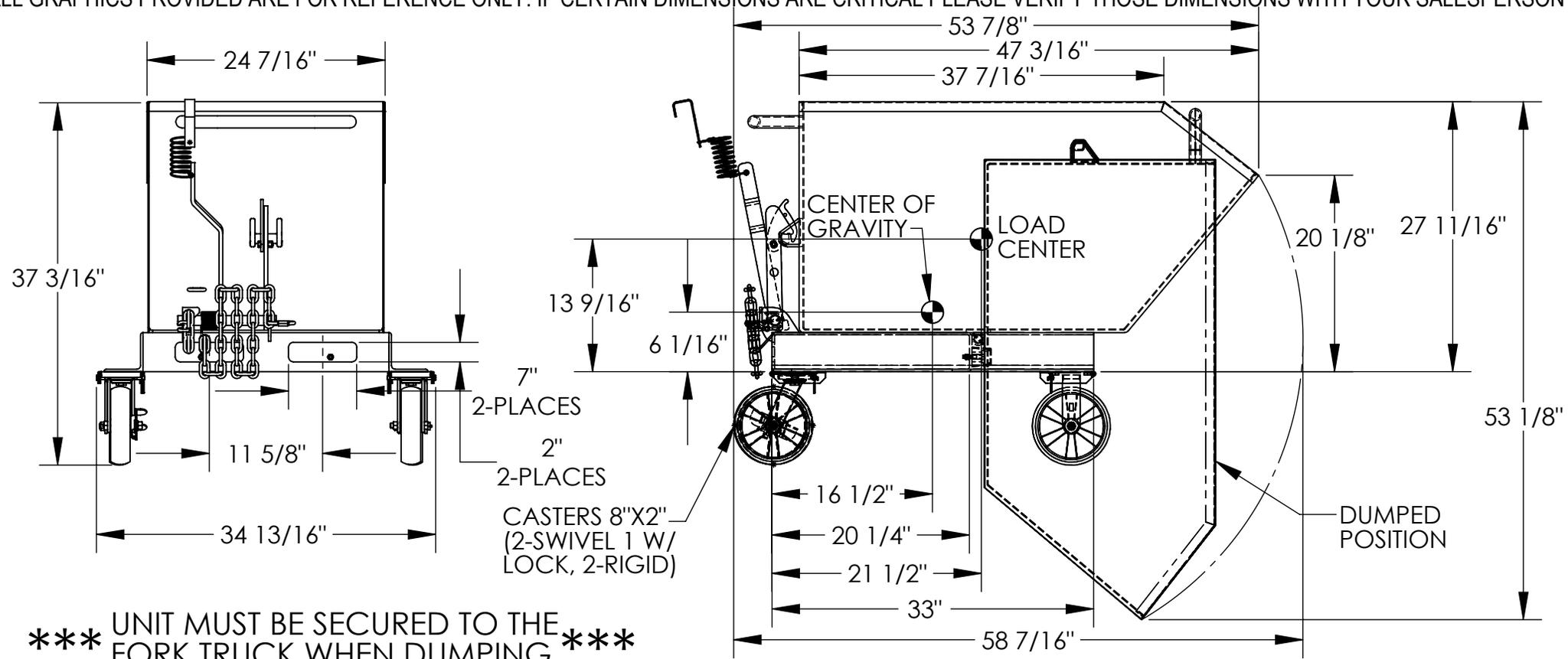
\*\*\* UNIT MUST BE SECURED TO THE FORK TRUCK WHEN DUMPING \*\*\*
