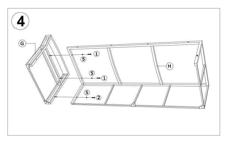
Locate Right backrest (I) to the Right base seat (H) and Right arm (G) by the pre-drilled threads. Use Allen Key (8) to fasten Bolts (1), Bolts (2) and Bolt (3) with Washers (5). Should have 7 bolts fastened. Only fixed bolts 50% (Photo 5).
