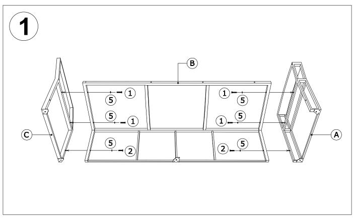
Locate Left backrest (D) to the Left base seat (B) and Left arm (A), Left small backrest (C) by the pre-drilled threads.
