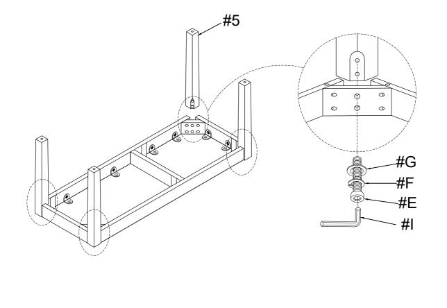
Do not tighten screws until completely asembled.
