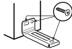
**4. Install the door panels.** Install the door panels by inserting the top pivot at the pivoting side of the door into the track bracket. Depress the guide pivot and position it under the track, then release it so the guide pivot is securely positioned in the track. With the top pivots inserted, lift upward on the panels and position the bottom pivot into the jamb bracket on the floor. Let the bottom pivot sit onto the jamb bracket firmly with the knurled teeth engaged.
