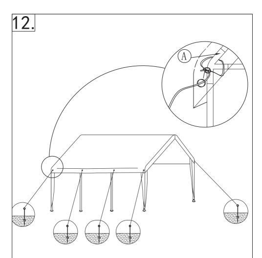
Fixed and tightened the 8pcs ropes ,and then the 4pcs sandbags filled with sand or soil tied in the four corners of the leg tubes.
