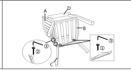
Attach Right Leg with Arm(C) to Backrest Panel(A) and Chair Seat Panel(B) using Bolts(1), and Bolts(2) with Allen Key(3).
