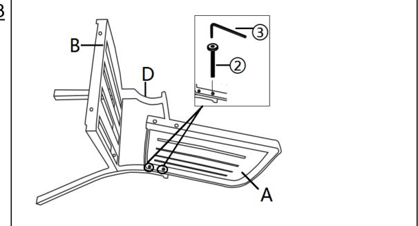
Attach Backrest Panel(A) to the Left Leg with Arm(D) using Bolts(2) with Allen Key(3).
