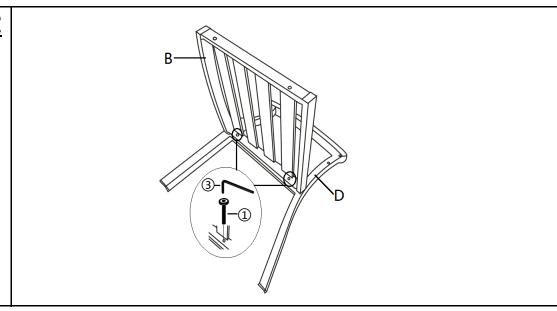
Attach Chair Seat Panel(B) to Left Leg with Arm(D) using Bolts(1) with Allen Key(3).
