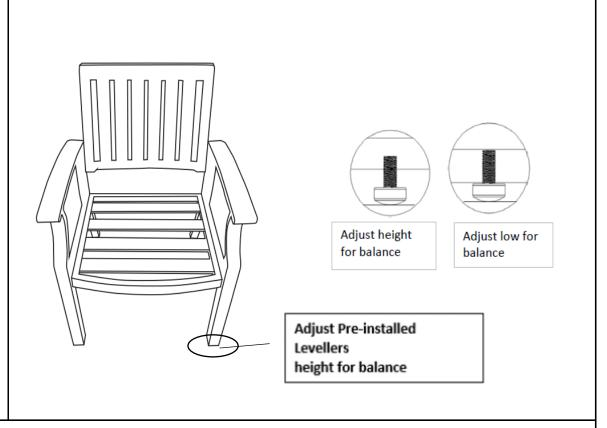
Adjust the Pre-attached levellers at the bottoms of the chair legs until the chair is level with the ground.
