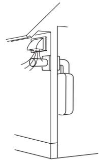
State of California: The water heater must be braced, anchored or strapped to avoid moving during an earthquake. Contact local utilities for code requirements in your area or call: 1-866-766-7489 and request instructions.
