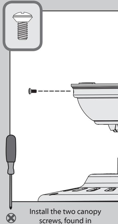
Install the two canopy screws, found in the ● hardware bag.
