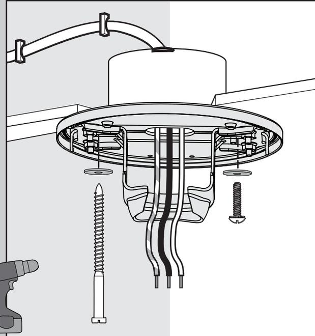
**Use wood screws** (included) and washers when securing to support structure with approved electrical outlet box. Drill 9/64" pilot holes in support structure to aid in securing ceiling bracket with hardware found in the ★ hardware bag.
