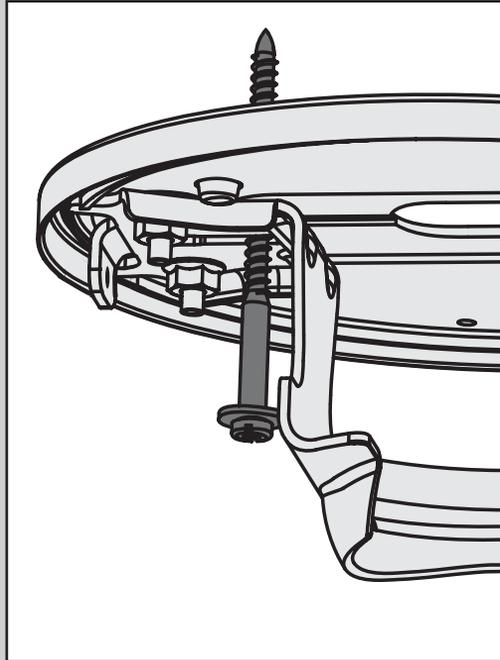
Use the wood screw to poke holes through the rubber gasket in order to install the ceiling bracket assembly to your support structure or ceiling fan-rated outlet box.
