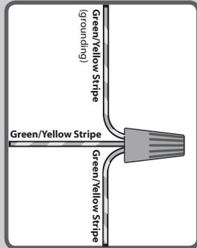
Using an orange wire connector from the ★ hardware bag, connect the 3 grounding wires (green, green/yellow stripe, or bare copper) coming from the ceiling, downrod, and hanging bracket.
