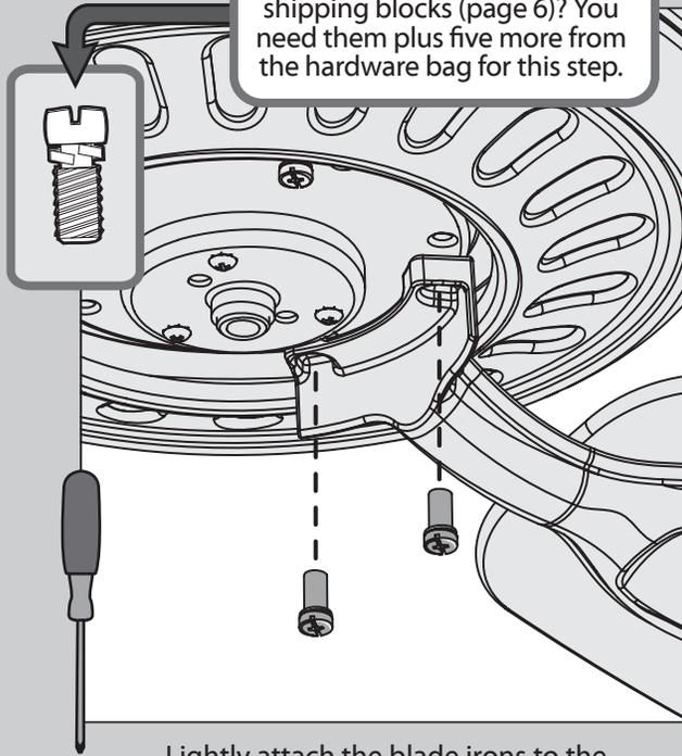
⊗ Lightly attach the blade irons to the motor with screws found in the X hardware bag, then securely tighten after both screws are attached.
