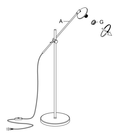
Assemble the Lamp Shade (F) to the lamp holder of Lamp Body (A) using Ring (G) to tight, then assemble Bulb (H) to the lamp holder tightly.
